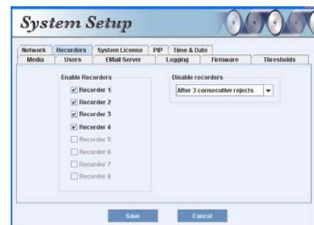
System will continue to run without using the disabled recorder. All recorders can be re-enabled at any time by selecting them within this tab. The number of consecutive rejects allowed prior to automatic-disable can be set to any number between 3 and 16 (inclusive). This feature can also be disabled by selecting 'Feature Disabled' in the 'Disable recorders' option.
